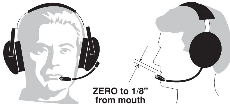
Figure 14 - Correct Positioning of Boom and Microphone
