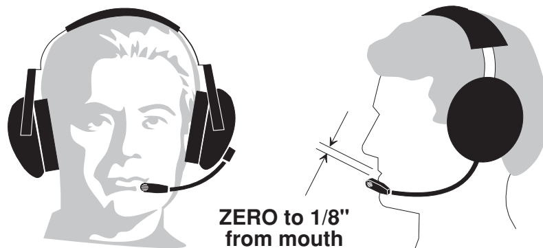
Figure 14 - Correct Positioning of Boom and Microphone
