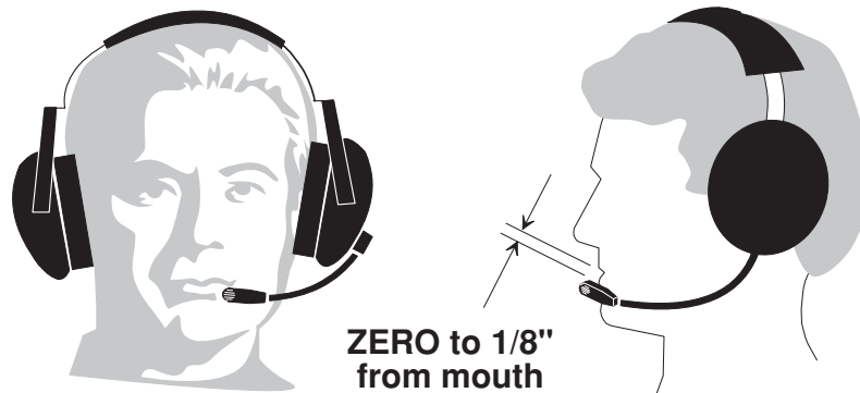
Figure 14 - Correct Positioning of Boom and Microphone
